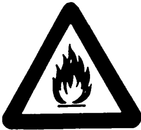
Flammable material or high temperature (1)
