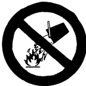
Do not extinguish with water
